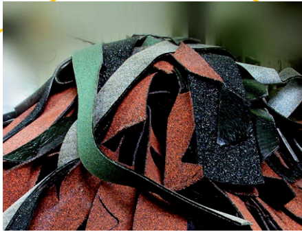
Collection of offcuts, production offcuts and old roofing membranes
