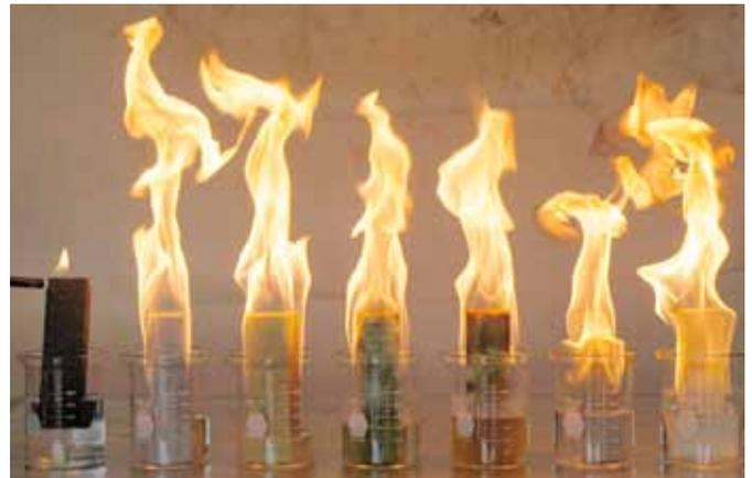
*Undeniable proof of fire safety in the wicking test. Flammable liquids wick through and soak insulation materials*
